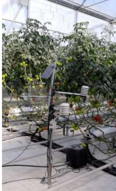
Figure 6. Temperature (°C), relative humidity (%) and solar radiation (W m -2 ) sensors installed inside a greenhouse compartment cultivated with a soilless tomato crop
